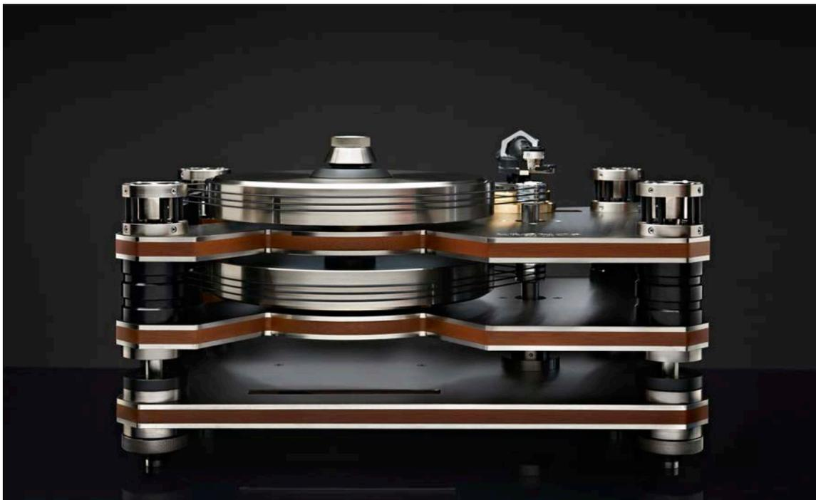
The entire platter system on the Kronos is floating, with twenty-four O-rings (a composite of three materials including Biton and Silicone) holding the weight. Each platter is engineered to eliminate vibration and is constructed in a “clam-shell” like fashion. Twenty-four fasteners force the top and bottom layers (made of aluminum) to compress the material inside (phenolic). Basically, the platter is a vice that squeezes itself to eliminate resonance.
