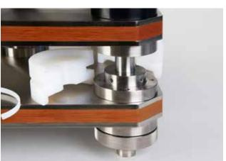
Remove the white leg spacers by cutting the tie wraps. Keep the spacers in a safe place, you will need them if you need to move the Kronos, or if you need to disassemble it for transport. Additional tie wraps have been supplied for such an eventuality. It is very important that the Kronos not be moved without installing the white spacers. Failure to do so could damage the speed sensors located left of the platters.
