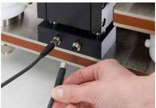
Connect the female end of the 2 pico cables to the motor base. Be careful as there is a **3 pin cable** and a **4 pin cable**.
