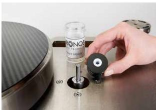
Install the top pick up pulley. Grease the pulley shaft and also grease the shoulder of the shaft assembly. Insert the pulley. **Do not over grease.** Once every 6 months or so, the pulley can be removed, cleaned (along with the shaft) and re-greased. This will insure better speed stability. Install the 3 belts as in step 10.
