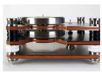
Carefully deposit the top platter (the one with the spindle) onto the bearing shaft. **The platter should rotate freely.** If it does not, remove the platter and make sure the ball is on top of the bearing shaft.
