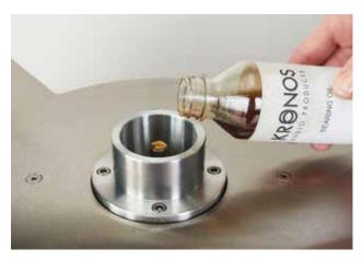
Add 8 ml. of Kronos bearing oil. Make sure the bearing shaft is oiled. A syringe is included in your kit to facilitate this process.
