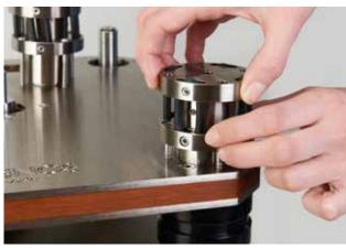
Slide in the 4 leg caps, making sure the socket head screws glide into their respective holes. Wiggle everything a little, the caps should find their way flush against the deck.
