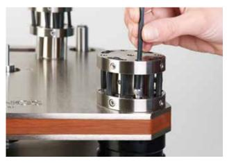
13 Tighten the socket head screws. Do not over tighten.
