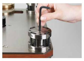
Level the suspended turntable by loosening the screws at the top of each leg (through the hole at the center top of leg caps). Level the turntable left to right and front to back. Tighten the set screws securing the leg caps to the leg shafts
