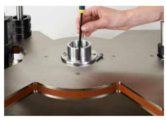
6 Install the silver colored bearing well using the supplied 10-32 socket head screws. **Do not over tighten.**
