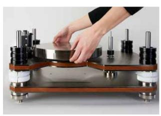
Carefully deposit the balancer platter (the one without the spindle) onto the bearing shaft. **The platter should rotate freely.** If it does not, remove the platter and make sure the ball is on top of the bearing shaft.
