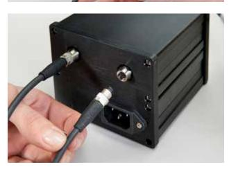
Connect the male end of the 2 pico cables to the power supply. Be careful as there is a **3 pin cable** and a **4 pin cable**. Connect the power supply to the AC mains. The power supply AC input voltage is set at the factory to either 110 volt or 220 volt. If a change of AC input voltage is required, please contact us so that you can ship back the power supply for a voltage change and re-calibration.
