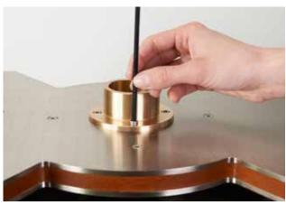
Install the gold colored bearing well using the supplied 10-32 socket head screws. Do not over tighten. Add 8 ml. of Kronos bearing oil. Make sure the bearing shaft is oiled. Place the bearing ball on top of the bearing shaft. Make sure it does not fall in the bearing well.
