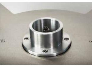
Place the bearing ball on top of the bearing shaft.
