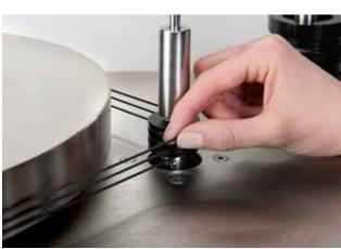
Install the 3 belts onto the motor pulley and pick up pulley. **Make sure no grease or oil contact the belts.** If this happens, the belts can be cleaned using regular glass cleaner.
